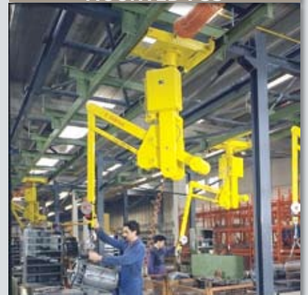
OVERHEAD TROLLEY MOUNTED PSS
